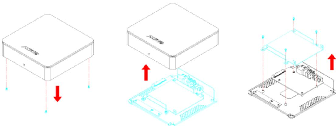
Install the hard drive in the HDD chassis and fasten the screws on the sides to hold it in place. Mount the HDD chassis and replace the top enclosure. Fasten the screws at the bottom of the case, place the rubber feet over the screws and stick them on the casing to cover the screws.
