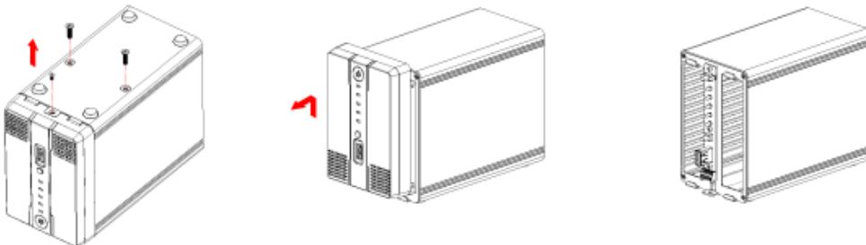
Install the hard drives as illustrated below with the top of the drives, where the label is located, facing each other. Push the drives lightly into place and then replace the front panel. Mount the front panel and the drives by fastening the screws at the bottom of the case.
